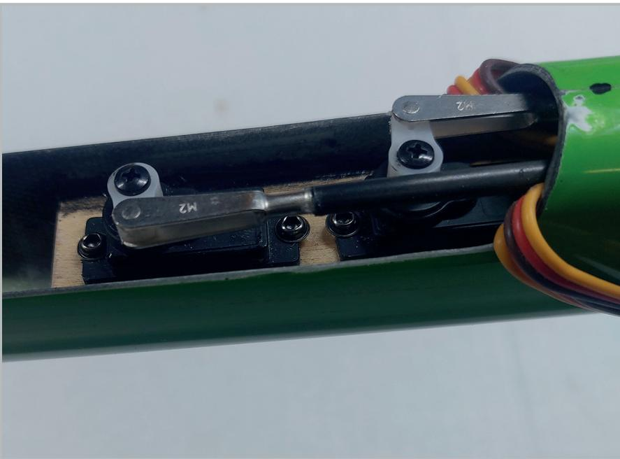
Now the servo board can be glued into the hull with the rods fitted. This results in the exact position in the fuselage boat.
