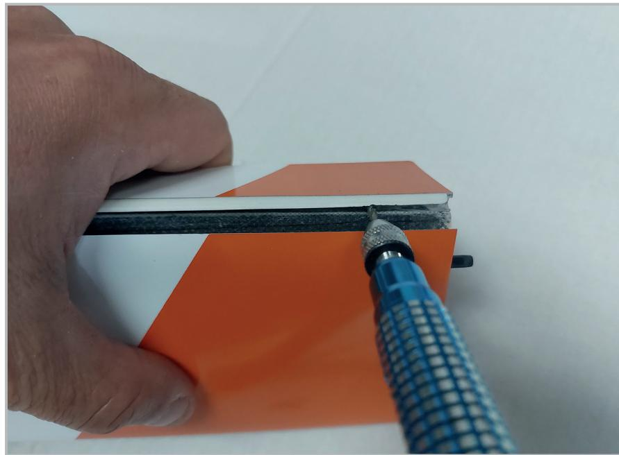
For this purpose the rudder blade is brought into a large deflection angle. ATTENTION: drill by hand! Do not damage the surfaces of the rudder.
