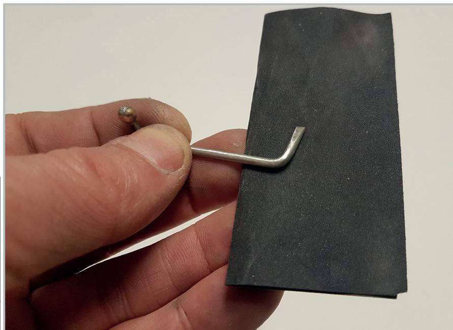
Now grind the two angled linkages a little bit flat to avoid damaging the surface in the rudder.
