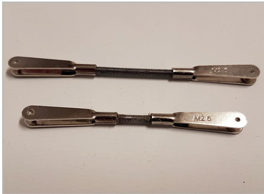
Make the aileron and flap linkages from the threads and the clevises, using screw locker.
