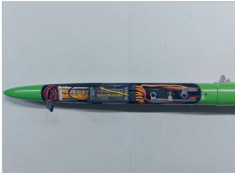
The receiver can now also be plugged in according to the manufacturer/system and installed well padded.
